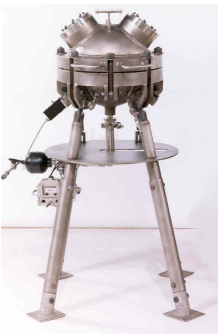
Figure 3: The 20-Litre Apparatus owned by the Fike Corporation is pictured here. Source: Fike Corporation, used with permission.
