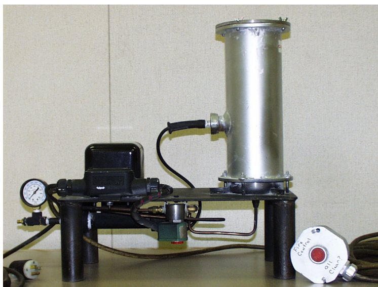
Figure 2: Pictured above is a simple version of the Hartmann 1.3-Liter Apparatus used for much of the early work by the U.S. Bureau of Mines to study dust explosions.
